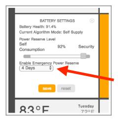
To maximize security for emergency backup, this level should be set a high percentage. A high power reserve percentage keeps the batteries toped off for emergency backup situations.
